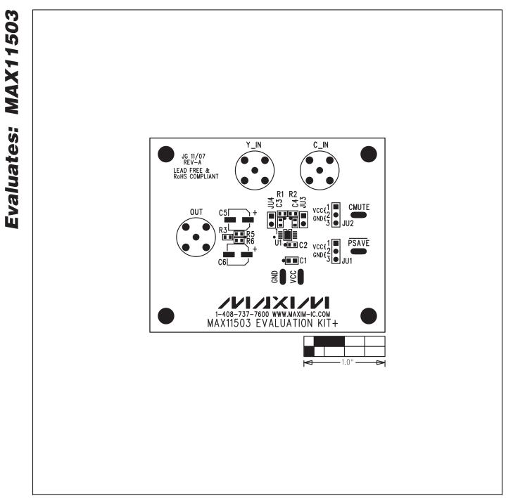
Figure 2. MAX11503 EV Kit Component Placement Guide—Top Silkscreen
