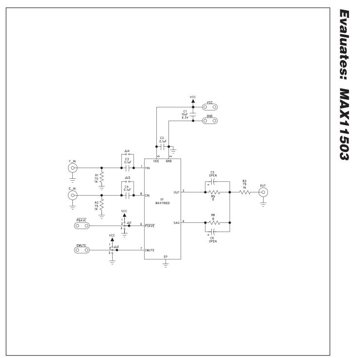
Figure 1. MAX11503 EV Kit Schematic
