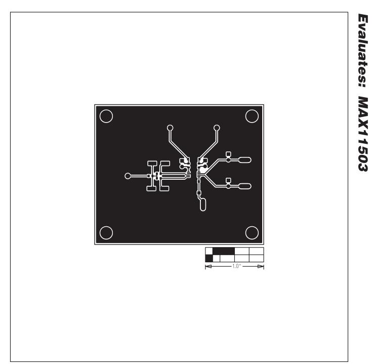
Figure 3. MAX11503 EV Kit PCB Layout—Component Side
